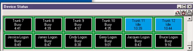
**Device Status:** Provides real-time status of devices on the system. The software can monitor and report on a wide variety of devices including analog trunks, T1 channels, PRI channels, trunk groups, ACD logon buttons, park zones and many others. Using information presented on the device activity screen, a supervisor can oversee and report on the system's incoming and outgoing call traffic as well as monitor agents that may be misusing certain features on the system.
