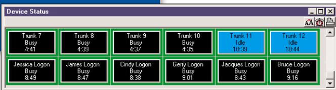
**Device Status:** Provides real-time status of devices on the system. The software can monitor and report on a wide variety of devices including analog trunks, T1 channels, PRI channels, trunk groups, ACD logon buttons, park zones and many others. Using information presented on the device activity screen, a supervisor can oversee and report on the system's incoming and outgoing call traffic as well as monitor agents that may be misusing certain features on the system.
